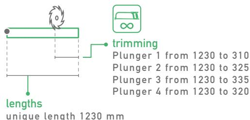
**EN** One of the all-time CCE classics, available with many different combination of seals and plungers, it guarantees a high efficiency. Its mechanism can be pulled out from both hinge and lock sides (CCE patent). This model can be installed also on pivoting doors in combination with Actuator Pivot accessory.
